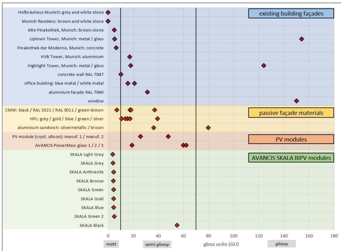
**Figure 4.** Gloss values of PV modules and façade materials as well as already existing building façades. CWM: compressed mineral wool, HPL: high pressure laminate. See subsection 2.1 for details on how data was acquired as well as an estimate of the measurement error of these values.
