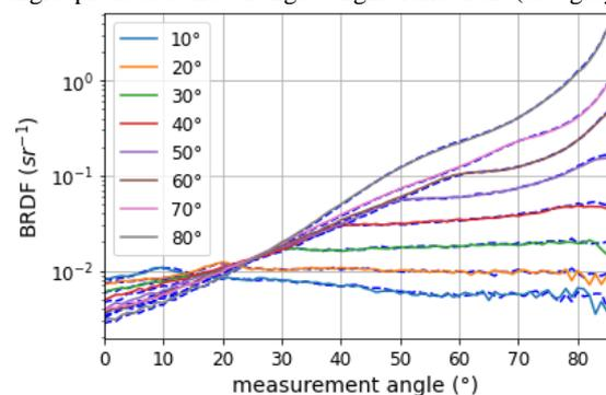
**Figure 7.** BRDF results for AVANCIS SKALA Green for two different sample orientations at incident angles ranging from  $10^\circ$  to  $80^\circ$  in  $10^\circ$  steps. Dashed lines represent the same measurements with the sample azimuth turned by  $90^\circ$  (see Figure 2).
