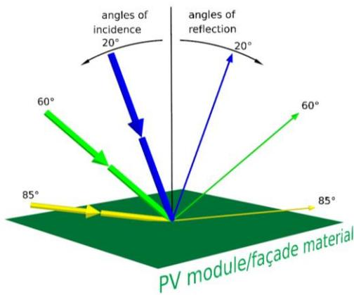
**Figure 1.** Angles of incidence and reflectance used in gloss measurements. Only specular reflection, where the angle of incidence equals the angle of reflection is assessed in this measurement setup.
