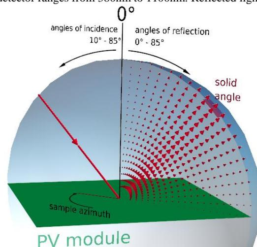
**Figure 2.** Geometry for 2D BRDF measurements: angles of incidence ranging from 10 to 85° while reflection is measured at angles ranging from 0 to 85° (for lab 1). The measurement is performed in plane with the light incidence.
