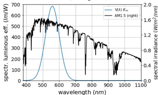
**Figure 3.** AM1.5 spectrum (in black) and the photopic spectral luminous efficiency function  $V(\lambda)$  (in blue) used to convert radiometric units,  $W/m^2$ , into photometric units,  $cd/m^2$ .
