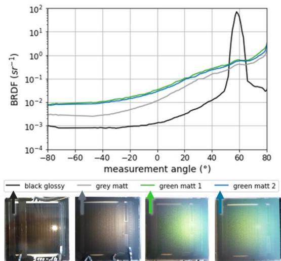
**Figure 6.** BRDF results at 638nm incident light wavelength and  $60^\circ$  incident angle for four different samples. The black curve represents the measurement on a module stack equivalent to the PV module AVANCIS PowerMax and the three other curves the measurement on modules stacks equivalent to the BIPV modules AVANCIS SKALA Colour (Grey, Green 1 and Green 2).
