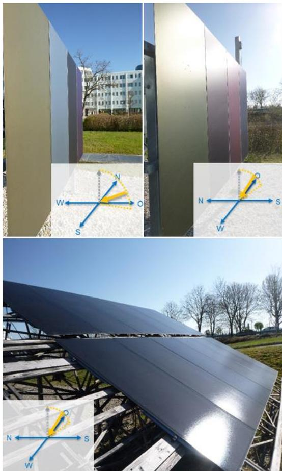
**Figure 5.** Pictures of various BIPV modules AVANCIS SKALA with incident sunlight at small angle to normal direction (top left) and at large angle to the normal (top right). As a comparison, roof-top PV modules AVANCIS PowerMax with incident sunlight at large angle to normal (bottom).
