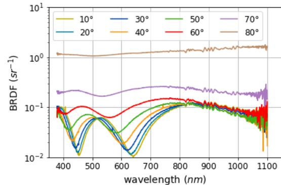
**Figure 8.** Spectrally resolved BRDF results in specular direction, i.e. where the angle of incidence corresponds to the angle of reflection.
